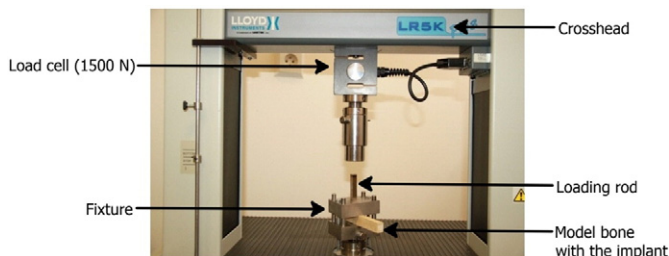
Fig. 5. The model bone in the fixture and loading in the testing machine.
